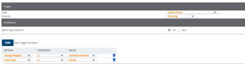
Figure 185: Example Hardware Monitoring Trigger Conditions
